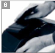
6 Bend E-Tube to remove lid
