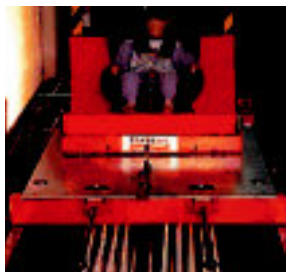
Crash test unit: 22 m/s speed and 784 m/s 2 acceleration, travel speed ► page 1.19
