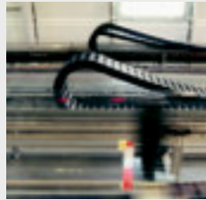
Push Pull forces speed up to 10 m/s, acceleration up to 200 m/s 2 are tested by igus®
