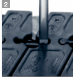
2 Tap gently to remove connectors
