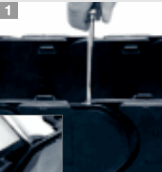
Remove crossbars, clips, and lids on two adjacent chain links. Guide the screwdriver into the slot between side links and release it by levering it and separate the E-Chain®
