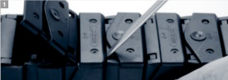
1 To open Series 352 and Series 353 only - Insert screwdriver into slot on top of lid and push down
