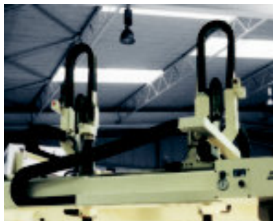
Standing application - R68 Tube - Note: the first links are supported
