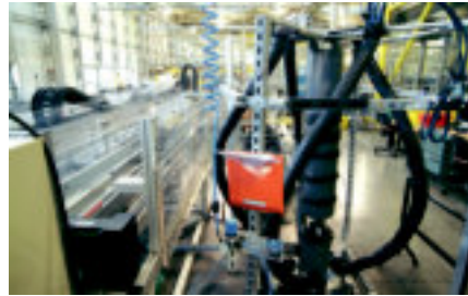
Component test - torsion tests for cables
