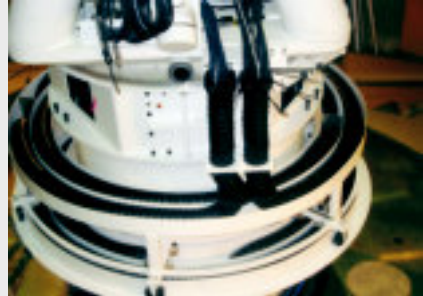
Laser measuring telescope with Triflex ® R. Rotary motion in both directions \leq 30^\circ . Also possible at high speeds \leq 20 m/s
