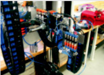
E2/000 dirt-insensitive E-Chain®, which saves installation space - here Machine tool for workpieces
