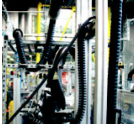
Torsion testing of Triflex® R in the igus® laboratory, Cologne
