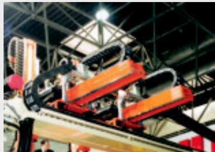
Machine tool gantry with various E4 E-Chains® - fast movements and high cycle counts
