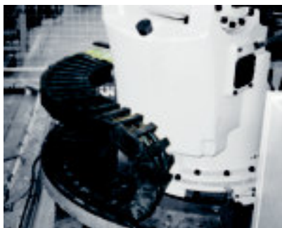
TwisterChain® for continuous industrial operation on a buckling arm robot (for welding applications, rotary movement 420°)
