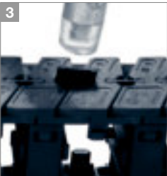
3 Gently reinsert connector by using hammer
