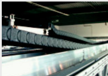
E-Chain® at the mast of the shelf conveyor rolls from one aluminum guide trough to the opposite one
