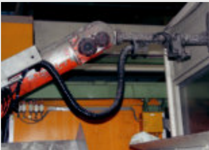
Triflex ® R in a magnesium die-casting industry (heat, dirt, oil, metal chips, dust, etc.)- failsafe
