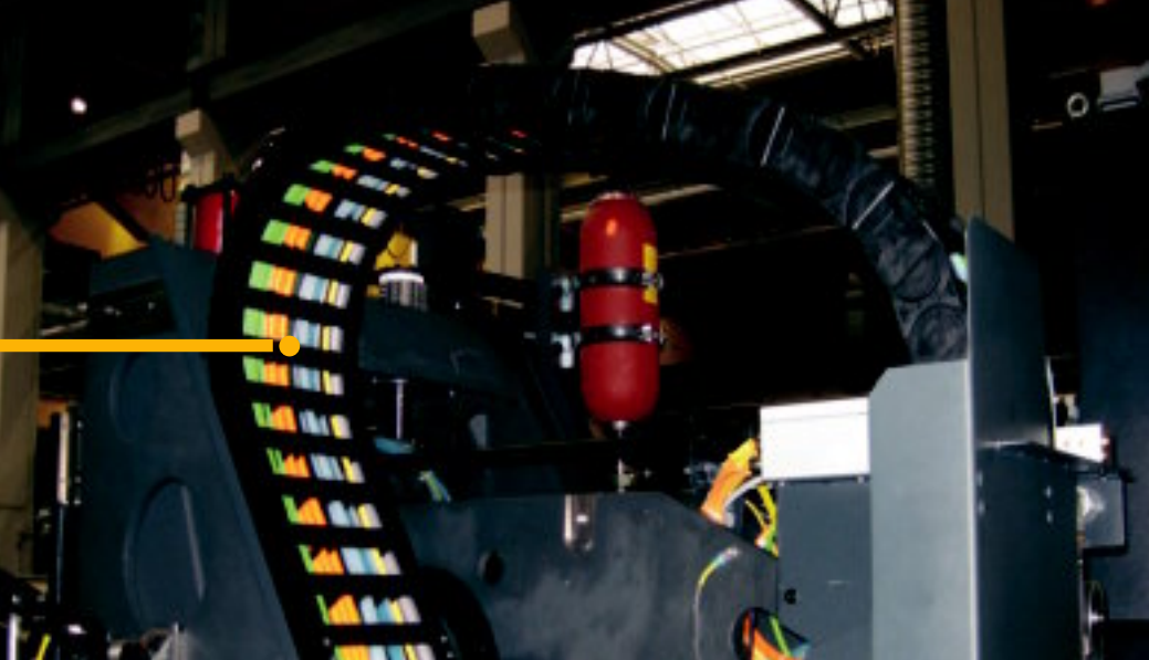
The E4.42 series in a machine tool, completely assembled with igus® Chainflex® cables
