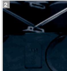
Remove clips - Insert screwdriver into the slot and push down, release by lever action
