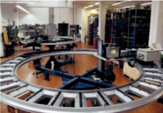
E2 mini E-Chain® as RBR-version with double bending radii
