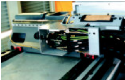
Machining center - System E4/light E-Chains®, Chainflex®-cables, metal parts and igus® strain relief
