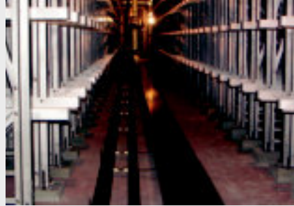
Long travel length with the super-alu-trough in a cold store
