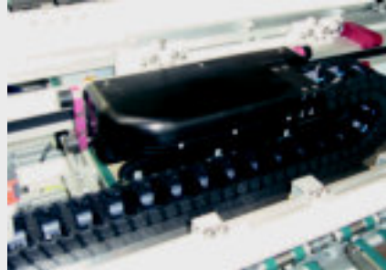
Serie E6 accelerates the work sequences in the case of this application for wafer handling. a = 4 \text{ m/s}^2 , v = 6 \text{ m/s}
