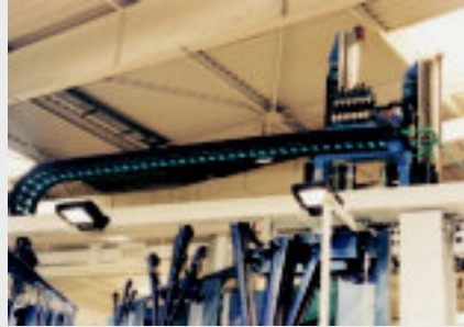
Unsupported application with harnessed E-Chain® System E4
