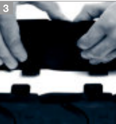
Join the side links together on the opposite side by applying pressure to the outer link
