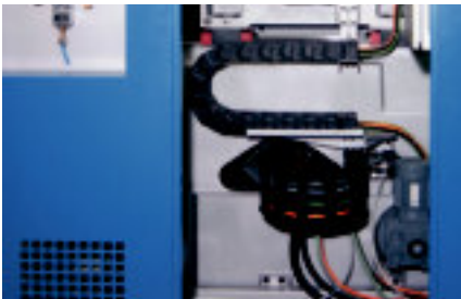
Horizontal machining center - harnessed with igus® E-ChainSystem® E4/4, Chainflex® cables and accessories
