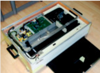
igus® Series E3.15 side mounted in a flat-bed scanner
