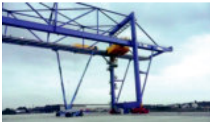
Successful application with P4.56 on a new RMG crane. 130 m travel length at 150 m/min speed. Harnessed with igus® Chainflex® motor-, control- and fiber optic cables
