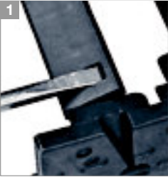
1 Lever crossbars with screwdriver
