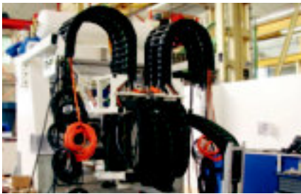
Machining center - System E4/light, Chainflex® cables, mounting plates and igus® strain relief systems delivered ready to install
