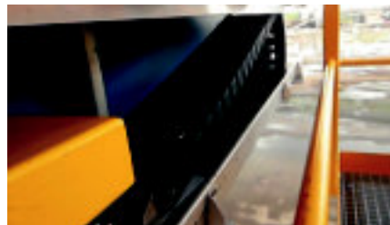
Successful application with P4.56 on a new RMG crane. 130 m travel length at 150 m/min speed. Harnessed with igus® Chainflex® motor-, control- and fiber optic cables
