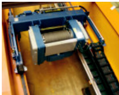
With the space-saving igus® E4 Polymer E-Chains® the overall dimension for the installation for this crane system was considerably reduced
