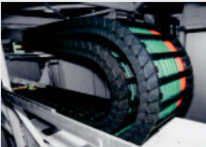
Nested E-Chains® reduce vibrations and improve milling accuracy Series E6.62
