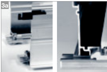
Fasten Basic assembly set Basic inside ③a or outside ③b (Check stability of the fixing). Please note: half the length of the assembly set and connector must protrude out of the trough. The glide nut should be well fastened in the C-profile
