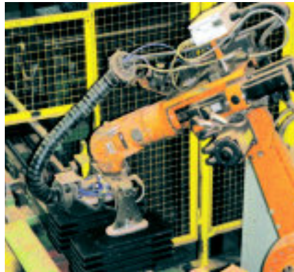
Optimal cable guidance even under extreme conditions, such as here in the Jungmeier roof tile plant
