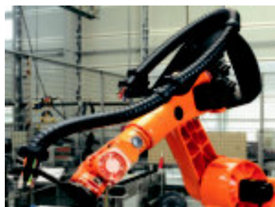
Triflex® R Set - Routed closely on the robotic arm for extreme flatness
