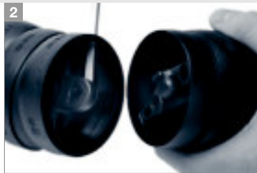
Insert screw driver into the opening of the socket from the top. Then twist apart, counter-clockwise
