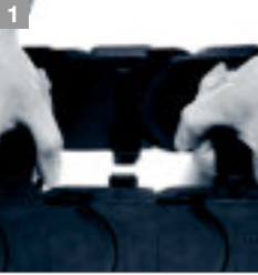
Remove crossbars at connection point. Slide side links into each other - Press together
