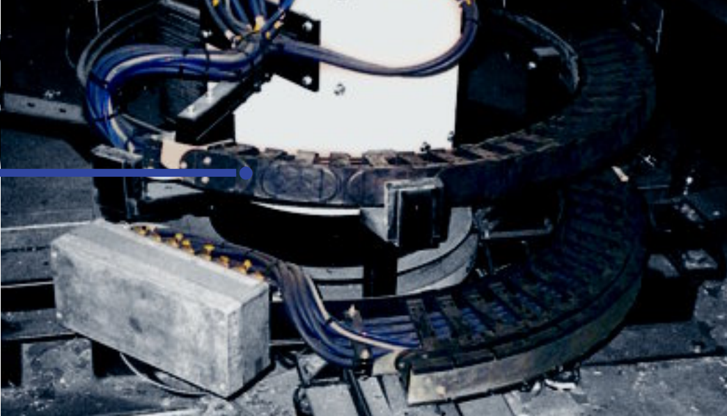
Combined spiral and rotary movement - igus® Series TwisterChain®
