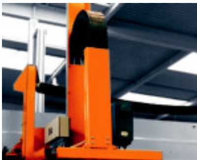
U-shaped supported E-Tube for high lateral acceleration
