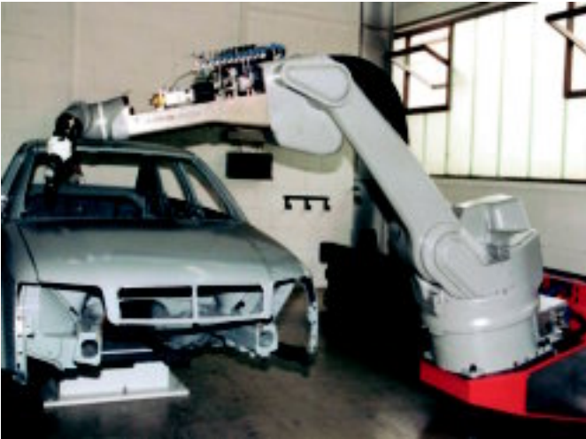
Spray-painting robot with System E4 E-Chain® used in an ATEX version made of igumid ESD. High accelerations of up to 6 m/s² and high braking rates with a weight of the robot of approx. one ton
