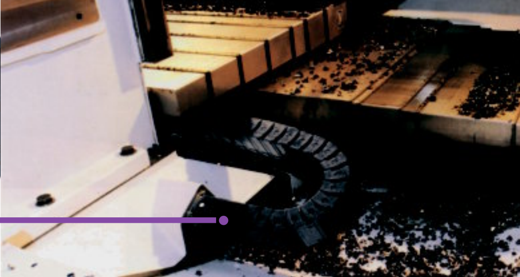
E2 E-Tubes in chip-area of a tooling machine. Resistant against hot metal chips up to 850°C
