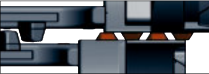
Offset operation of upper and lower run, resulting in continuous roll-through surface
