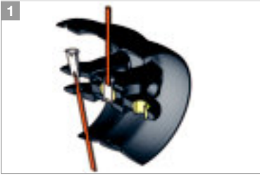
Connector principle = Ball head clevis joint (similar to the proven trailer hitch design) Improved assembly/disassembly for large sizes. Faster assembly with less effort
