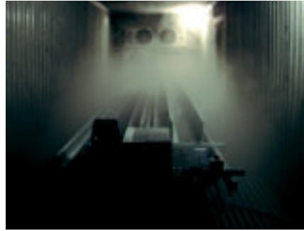
igus® climate chamber - E-Chain® and Chainflex® test runs possible at -40^\circ ( -40^\circ\text{F} ) to +60^\circ\text{C} ( 140^\circ\text{F} )
