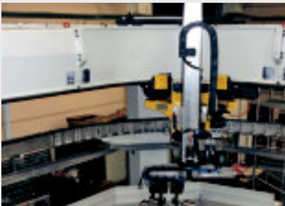
E4 E-Chain® was used here in curved sections with a 45 m travel distance
