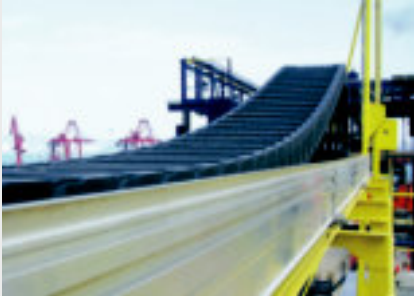
Seawater resistant super-alu-trough in a RTG-crane. Long travel with the E4/4 system
