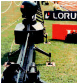
Mobile camera, Olympic Games in Atlanta, S = 100 m, v = 10 m/s in push-pull operation
