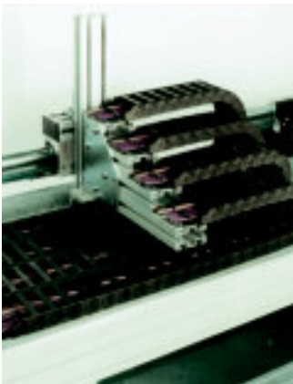
Example from igus® test laboratory: continuous development and testing of Chainflex® round electrical cables
