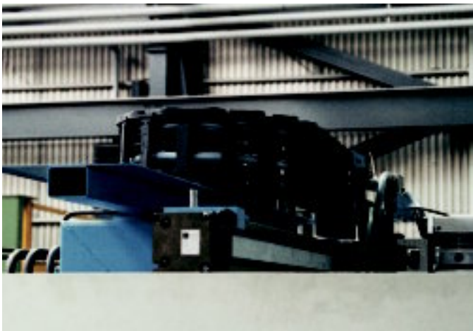
E-Chain®, side-mounted, supported System E4
