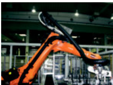
Fiber rod module for directed pretension and universal assembly kit for multifaceted adjustments
