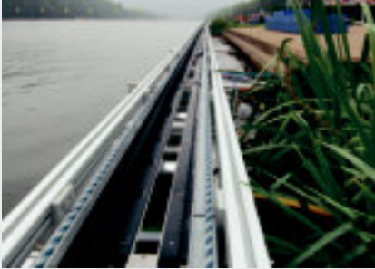
System E6, side mounted, in high-speed camera positioning system - high speeds and less vibrations
