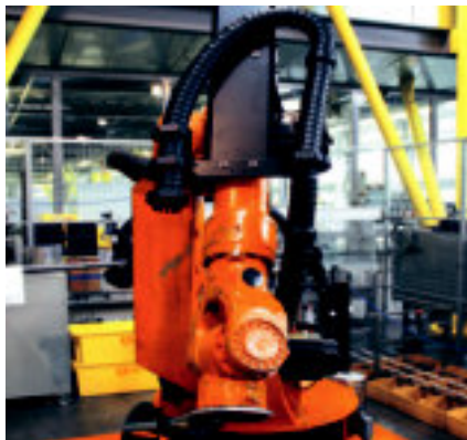
Integrated recuperating spring prevents loop formations
