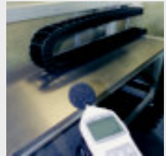
Noise level test inside an igus® acoustic cell
