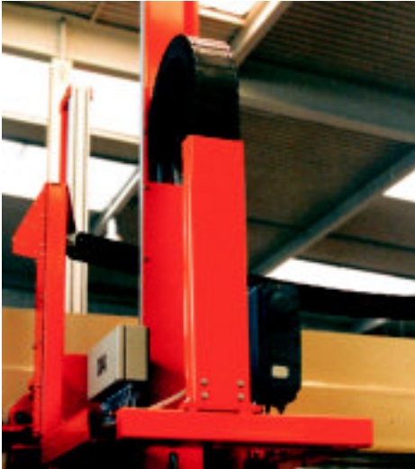
U-shaped supported E-Tube for high lateral acceleration
