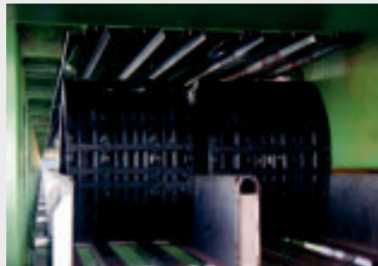
System E4 with extension link at a ship loader for the coal unloading Travel 105 m, speed 240 m/min, load 53 kg/m
