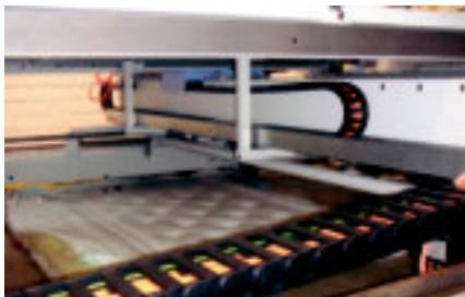
Harnessed igus® E4 E-Chains® on an X/Y unit in the textile industry with high cycle counts
