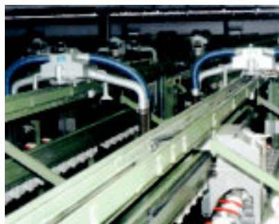
Long-travel applications up to 40 m are possible - here: Series 10 in textile machine
