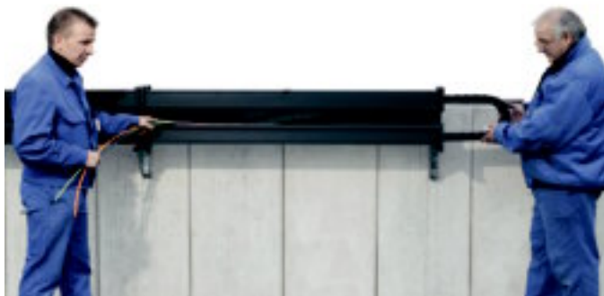
The installation variant of a floating moving end for compensating for any lateral offset tolerances between scraper and E-ChainSystem®
