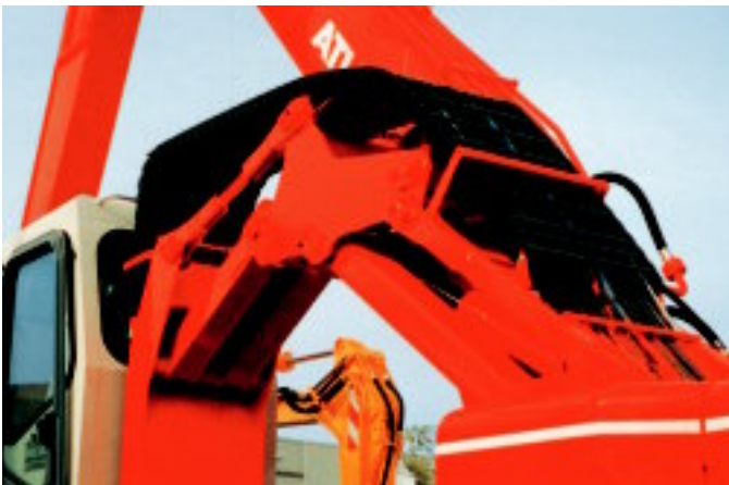
Combined horizontal and vertical movements
