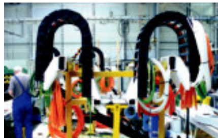
igus® ReadyChain® on mounting frames for lightning fast final assembly
