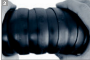
Hold two pieces together at inner radius and move socket up against the ball's wedged end
