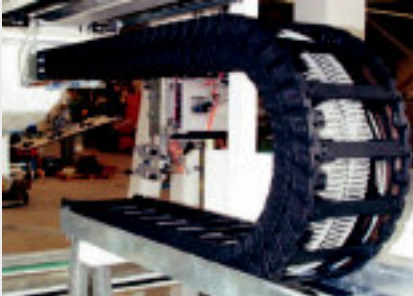
System E6 in a pick and place robot. Handles injection molded CD covers in a split second
