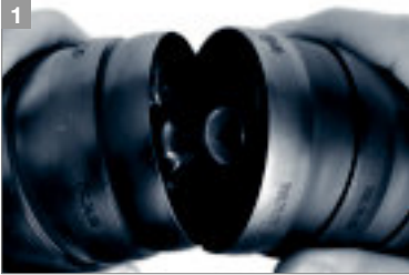
Hold two pieces together at inner radius and move socket up against the ball's wedged end
