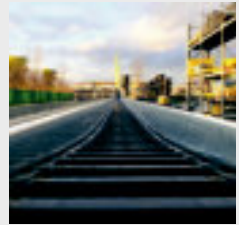
Long travel test field: 125 m travel length, speed 300 m/min
